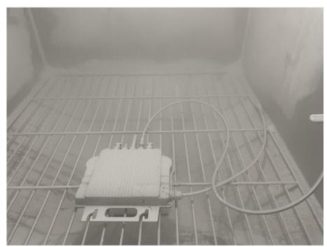
Test setup of IP6X
