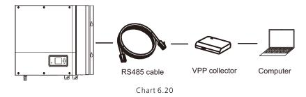
The external VPP collector is connected to 485-1/485-2 port through a network cable, at this time SPA will respond to the relevant instructions issued by VPP.
