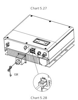
Note: If you are using a lead-acid battery, you do not need to install this communication cable.
