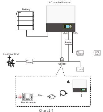
As shown above, a complete grid-connected system of SPA consists of SPA inverter, battery, utility grid and other components.
